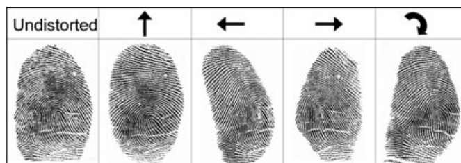
FIG. 2—Still images representing different types of distortion. The arrows show the directions of the applied forces.
